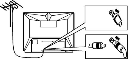
Note: In case of using the Twin-lead aerial feeder  $(300\Omega)$  for UHF/VHF aerial, use a 300-75 ohm adaptor (not supplied)
